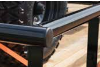
Pipe top rail and channel tongue design for improved durability.
