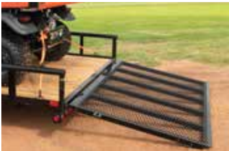
4' tall spring-loaded rear ramp gate for easy loading.
