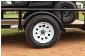
American-made Dexter Axles with low-maintenance EZ Lube Hubs.
