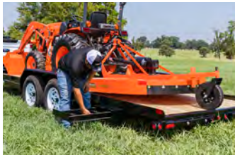
Stowable slide-in ramp package allows great versatility when loading equipment.
