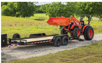
Low-profile angle iron frame for easy loading.
