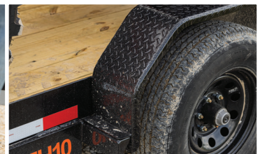
Heavy-duty diamond plate steel fenders are durable and strong.
